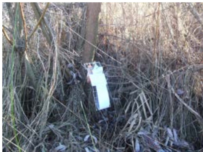
Fig. 2. Design of the hair-trap used in this study placed in a tree trunk. The adhesive tape was partially removed to allow observation of the structure; it usually covers the entire surface of the larger wire mesh piece.
